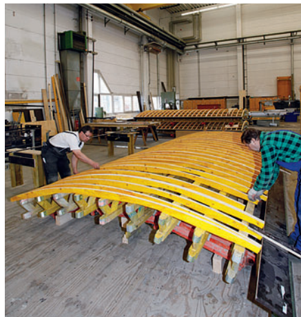
Assembly of GRV panels with segment boards.
